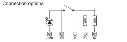
On the back of the call point there are 5 screw terminals connected to the internal PCB. Depending on where the wires are connected, the call point provides a series resistor, activates an internal LED or can simply provide a closing contact. If you choose to connect the +IN cable to the terminal marked +LED the call point, when operated, will switch on the internal red LED. Alternatively if you connect to the NO terminal the LED will not operate.
