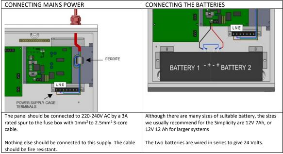
Once all the installation has been checked for any cable faults, and all the devices have been addressed and fitted, connect the loop and turn the panel on.
