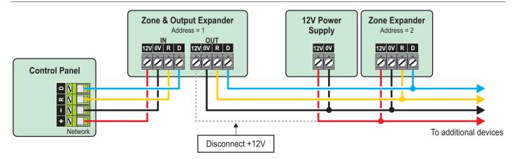
Remote keypads and expanders are all connected to the same network terminals located at the bottom left hand corner of the control panel and may be connected serially (daisy chain), in parallel (star) or any combination of the two.
